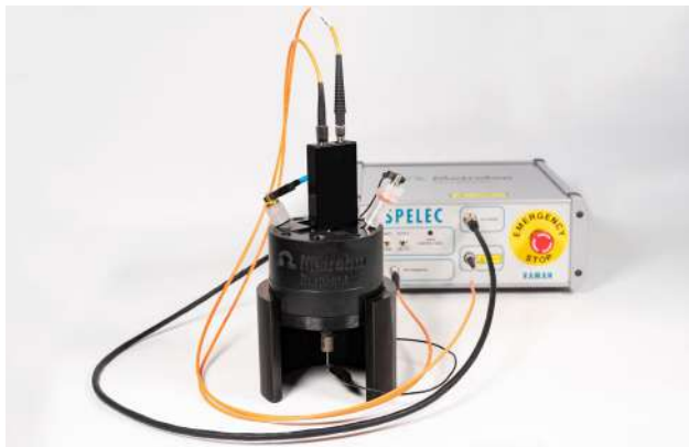
Figure 1. SPELEC RAMAN instrument and Raman probe used in combination with a Raman spectroelectrochemical cell for conventional electrodes.
