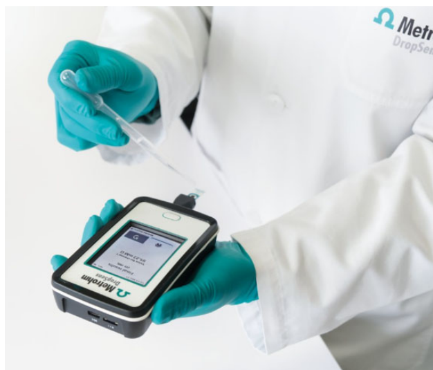
Figure 5. Example of a novel handheld setup where a miniaturized ion-selective screen-printed electrode is utilized with a portable potentiostat to make on-site measurements.
